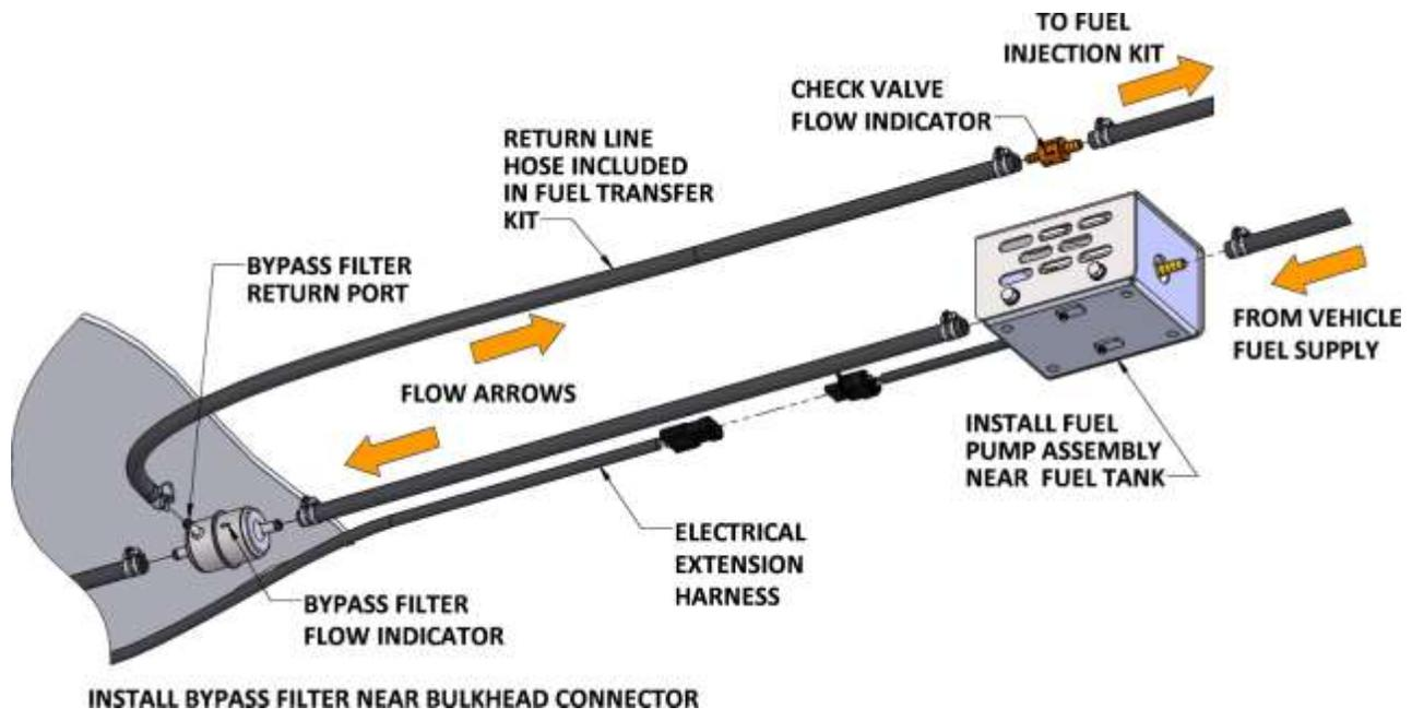
**NOTE:** Legend Brands uses a .0625" size bypass orifice fuel filter to achieve the correct fuel pressure. Using a fuel filter with a larger or smaller bypass orifice will not deliver correct pressure and can cause damage to the engine. To always ensure you have the right filter, we recommend only using the Napa Gold 3054 filter which can also be purchased directly from us with Legend Brands part number 36-212.
