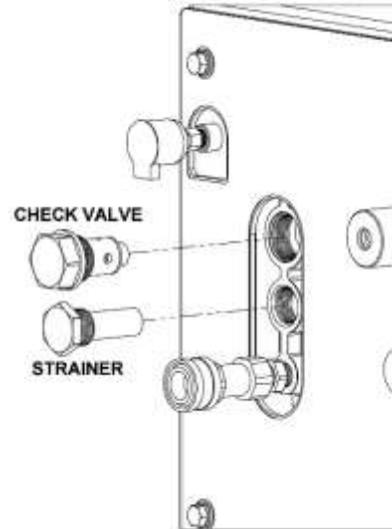
**NOTE:** New o-rings must be installed **anytime** the check valve is removed.
