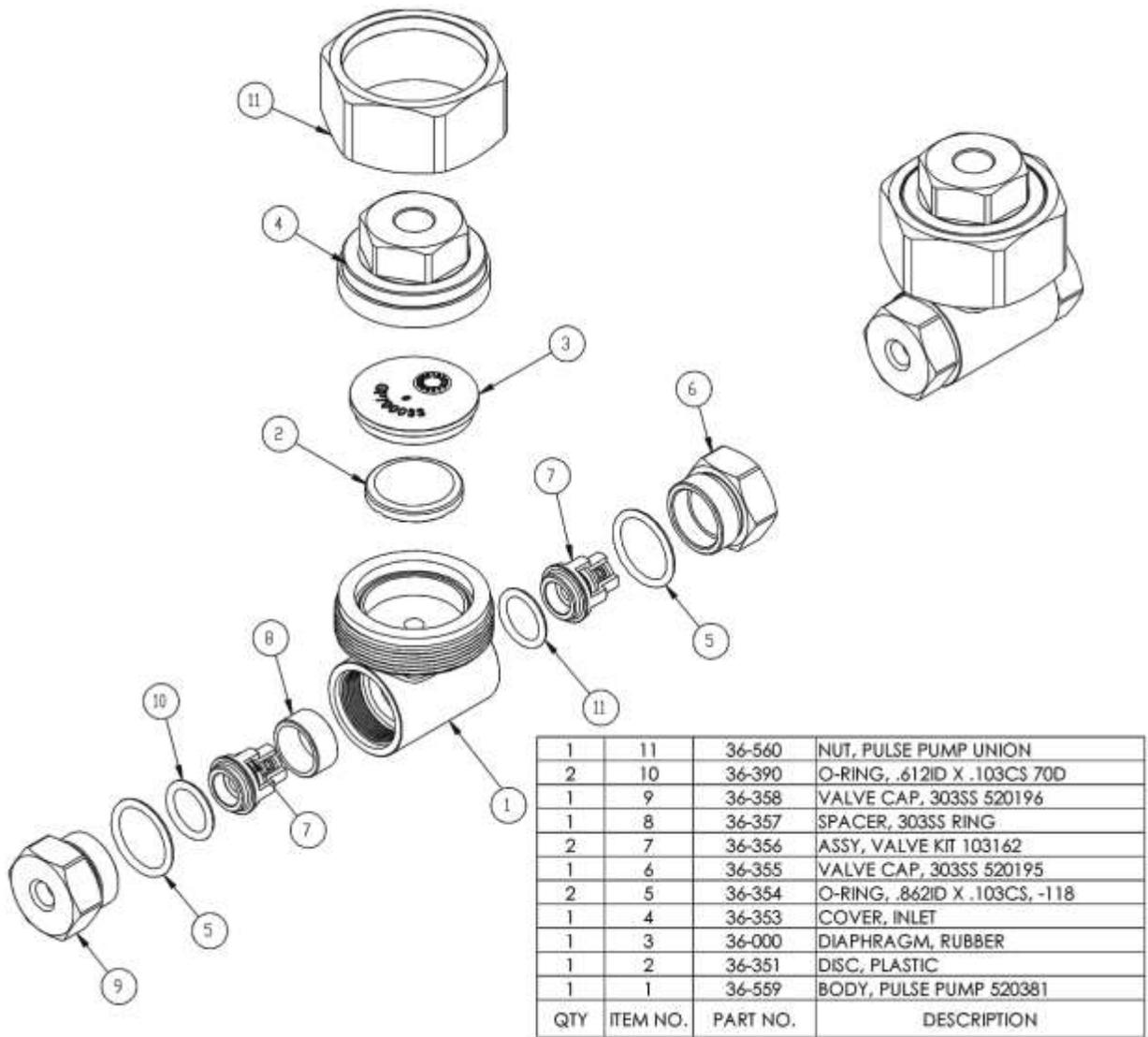
**SOLUTION MANIFOLD CHECK VALVE AND STRAINER**
