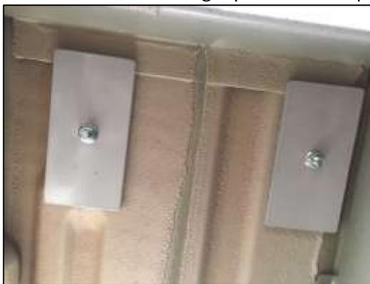
Screw the provided 3/8-16 hex head lock nuts on to the mounting bolts and tighten until the console and waste tank are firmly attached to the vehicle floor.
