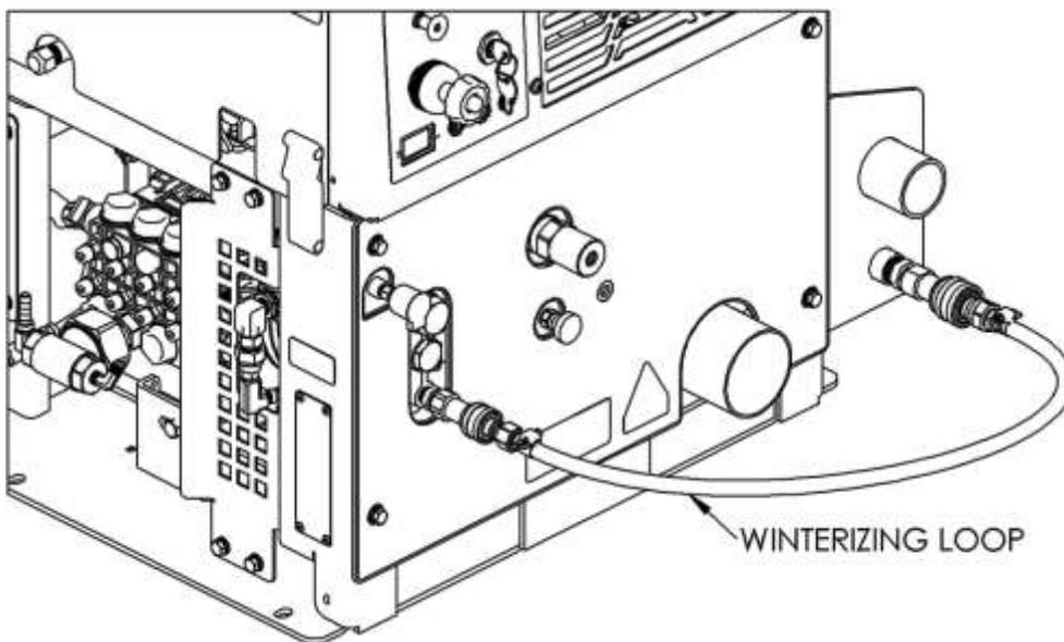
5. Turn the pressure regulator all the way down. Start the unit in idle, turn the Solution Pump switch to the ON position and run coolant through the system. Allow the unit to run for about 3 minutes to fully circulate the anti-freeze.
