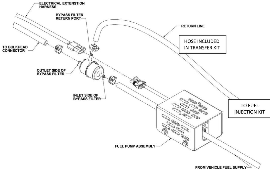
Figure 3. Fuel Pump and Filter Detail
