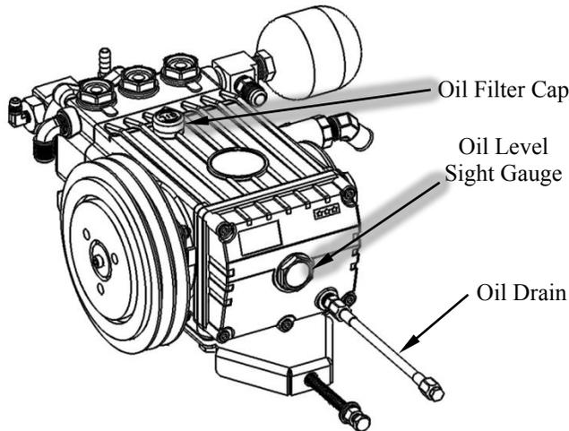
2. After the first **50 hours** of operation, change the crankcase oil with Industrial Pump Oil, (Part # 13-030). Change the crankcase oil every **500 hours** thereafter.
